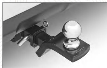
Trailer Hitch. Heavy-duty rated at up to 3,000 lbs towing capacity and 200 lbs tongue weight.
